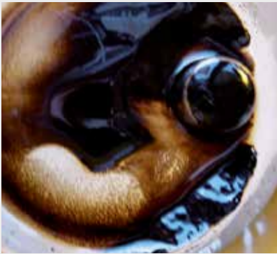
Poor thermal stability Significant deposits
