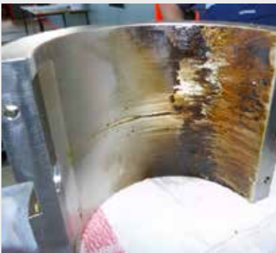
Deposits on bearing material
