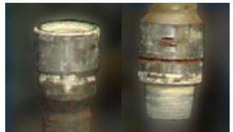
Figure 6 Connection after break-out
