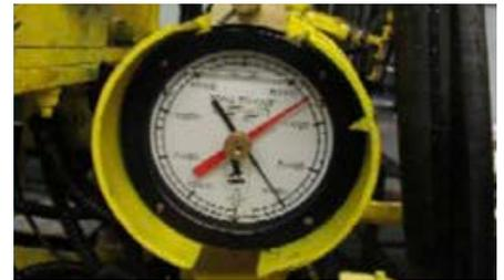
Figure 5 Torque at 90000 ft-lbs
