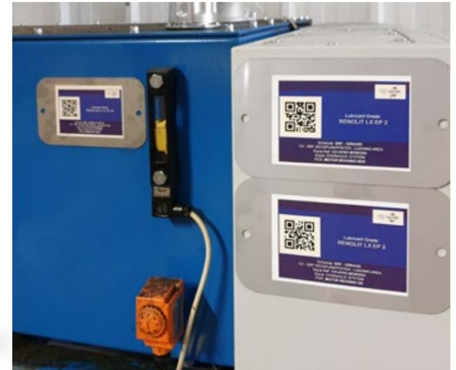
FluidsConnect uses QR code scanners to record machine specific content.
