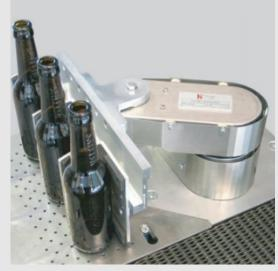
Above: The 3-axis servo pusher mechanism. This mechanism is responsible for transporting the glass containers to the conveyor system as seen in the picture below. This mechanism contains the bearings & chains which are lubricated with the NYE UNIFLOR 8623.
