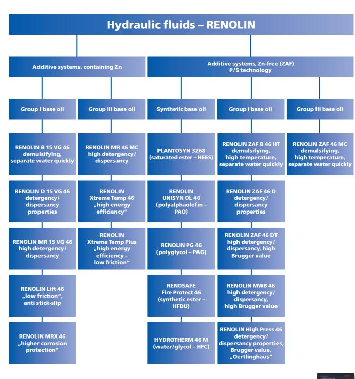
Example: ISO VG 46, kinematic viscosity 46 mm<sup>2</sup>/s at 40 °C
