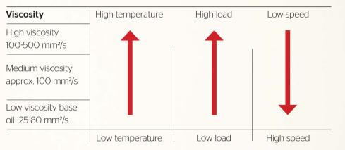
There are however exceptions when it comes to guidelines for base oil viscosity. Greases based on the NovaWay technology does not follow the common rules and experiences of conventional greases. Read more about this in the final lesson.
