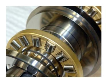
Among others, RENOLIN UNISYN CLP and RENOLIN UNISYN XT were used are used as high reference oils. With the RENOLIN UNISYN CLP 100 and RENOLIN UNISYN XT 100 high reference industrial gear oils, a test duration of > 9 million revolutions was reached in this roller bearing test without any WEC-type damage occurring.
