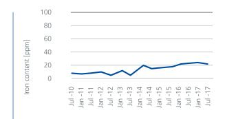
The test results of the used oil analysis prove the robust behaviour of RENOLIN UNISYN CLP 320 in main gear boxes of wind turbines of up to 8 years use!
