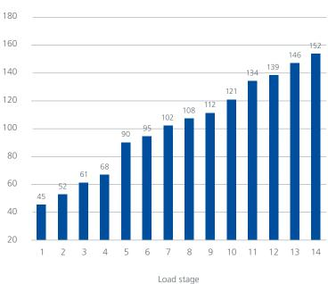
Example wind turbine 2 MW Test result with used oil sample: Failure load stage >14 - excellent scuffing protection
