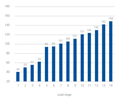
Example wind turbine 2.4 MW Test result with used oil sample: Failure load stage >14 - excellent scuffing protection
