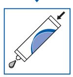
Depending on how the cartridge was filled, a small quantity of air may betrapped in the area of the screw thread.
