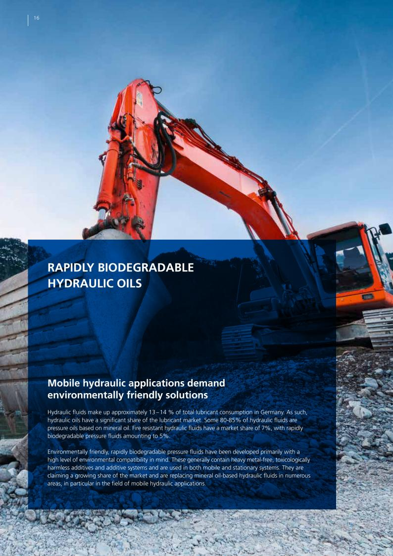
The minimum technical requirements of rapidly biodegradable pressure fluids are described in DIN ISO 15380.
