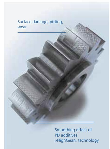
Both mineral oil-based and polyalphaolefin-based products are thus available which fulfill the highest technical standards. The results of tests performed in extreme conditions and with pre-damaged machine elements in large-scale gearboxes (in underground mine conveyor drives) as well as spindle drives in forging presses confirm these outstanding characteristics.
