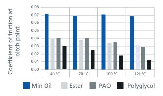
Accept additive packages more readily than mineral oils, and their refining process allows them to retain natural anti-oxidants and sulphur compounds with anti-wear characteristics.
