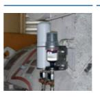
The 6-bar pressure generated allows for mounting at a distance of up to 5 m
