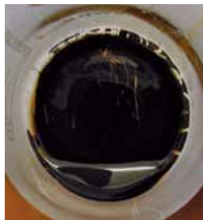
Competitor product (PAO-based): Poor thermal and oxidative stability
