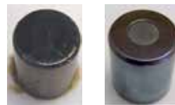
Competitor product (PAO-based): Poor thermal and oxidative stability
