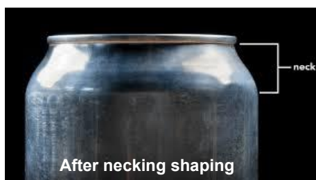
Beverage can neck forming process
