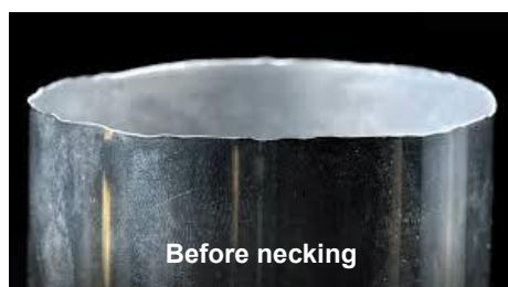
Beverage can neck forming process
