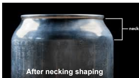
Beverage can neck forming process
