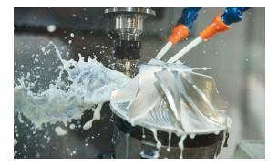
Proper coolant control – minimize flow rates and pressures
