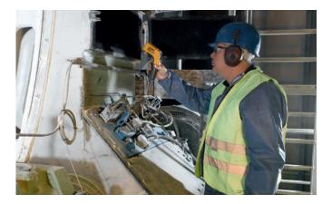
For drive units lubricated with CEPLATTYN GT, our service engineers carry out regular inspections throughout the entire service lives. They inspect the general operational status and check the spray system. In addition, the service engineers take extensive measurements (vibration, toothflank temperature) and carry out dynamic checks by infrared video thermography.
