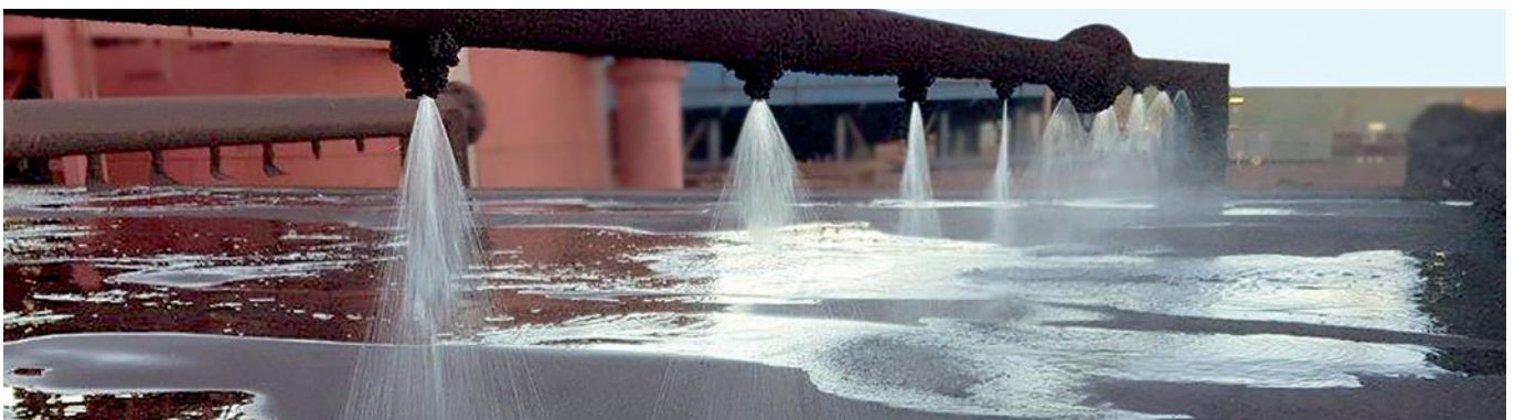
Spray bar configured to maximize cake moisture management
