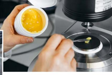
Preparations for a rheometer analysis to ascertain the properties of the lubricant. The smaller picture shows the second, rotating plate in its start position for the measurement. Then the black cover is lowered, meaning that you can no longer see the measurement plates. The cover ensures that the temperature can be regulated to predefined values.
